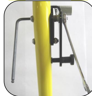
Ensure the device springs back freely, if it is too tight loosen M6 nut slightly
