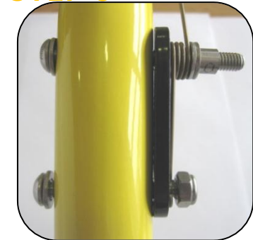
Insert 2 M6 washers and a 6mm Spacer
