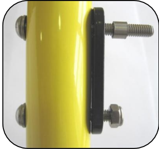
M6x45 bolt already on frame, insert M6x60 Bolt, washer and 6mm spacer
